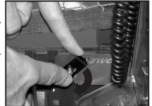
**7** Pull straight up on the robot body to remove it from the Center Trough. You may keep your old robot body, there is no need to return it to Newgy.
