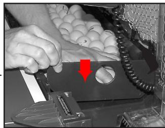
**4** Unhook the robot from the table and place the robot on top of the table. Place it with the robot facing you for easy access.
