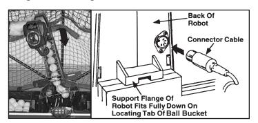
Reinsert the Connector Cable into the robot. Pull out the Ball Dam to release the balls so they roll back into the Center Trough. Reposition and reattach the Trap Net and Side Nets.
