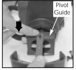
ATTACH CONTROL LEVERS Take the Right Control Lever and place its smaller round hole over the top post of the Pivot Guide. Be sure the opposite end of the lever is resting in the #1 slot of the Adapter. Now, do the same with the Left Control Lever, except make sure it is resting in the #6
