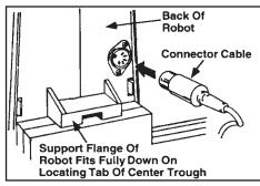
Reinsert the Connector Cable into the robot. Pull out the Ball Dam to release the balls so they roll back into the Center Trough.
