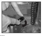
Pull straight up on the robot body to remove it from the Center Trough. You may keep your old robot body, there is no need to return it to Newgy.
