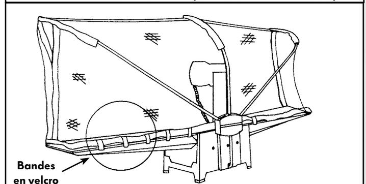
**IMAGE 15** AJUSTEMENT DE LA TENSION DU FILET PRINCIPAL (2055)
