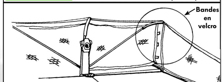
**IMAGE 16** AJUSTEMENT DE LA TENSION DU FILET PRINCIPAL (UNIQUEMENT 2055)
