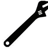
Adjustable Wrench (2.5" reach, minimum 1.5" Jaw)
