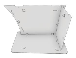
Place the back wall onto the base and screw it to the left wall and base.
