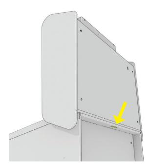
Using two people, set the backglass onto the table. Make sure the tab on the backglass fits into the slot in the table.
