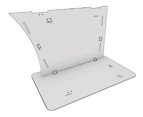
Place base (Panel E) on floor with grooves facing up. Place left wall into slots on base and use bracket to screw together.
