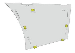
Locate the left wall (Panel A). Screw five (5) brackets to the inward facing side (side with slots).
