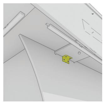
Under the front of the table, add brackets to the right and left sides. You may need to slide the front of the table around a bit. TIGHTEN THESE SCREWS LOOSELY.
