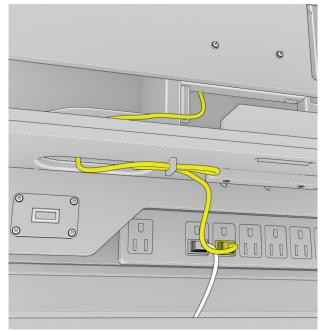
Locate the power cable for the backglass monitor. Carefully cut the zip tie. Run the cable down through the slot and plug into power strip. Bundle excess cable in the clip.
