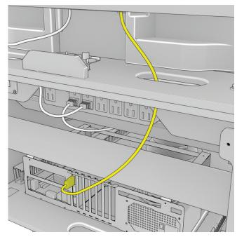
Locate the HDMI cable for the backglass and run it down through the slot. Attach it to the top port on the graphics card.
