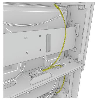
Locate the marquee cable on the floor of the table. Plug the middlet connector into the circuit board and the other into the marquee connector.
