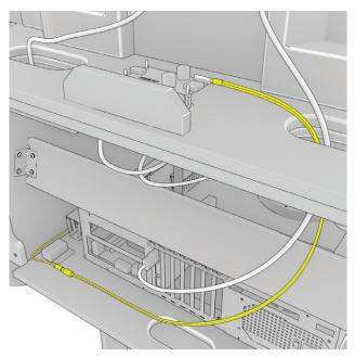
Locate the audio cable bundled to the bottom of the backglass (looks like a thick, black, double cable). Run it down through the slot and attach to the audio jack on the lower left of the table.
