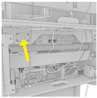
There is a DEMO MODE switch to the left of the power strip. Turn this off (circle down) unless you're setting up for a retail display. Finally, put the rear panels back onto the backglass and table.
