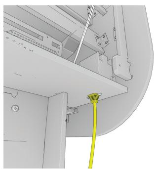
Attach the power cable into the plug under the right outlet box.
