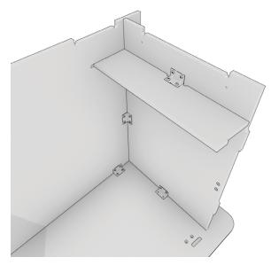
Place rear brace (Panel H) into slots on back and side walls. Slots will face down. Screw to bracket.
