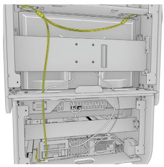
Locate the speaker cables on the bottom of the table (Looks like four cables bundled together with square plugs).
