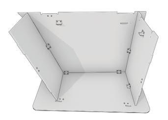
Place the front wall (Panel D) onto the base and screw it to the left wall and base.
