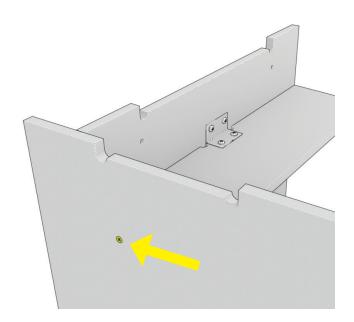
Add a BLACK screw to the rear brace from the outward facing side of the left wall.
