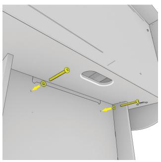
Use two (2) bolts and two (2) washers to secure the rear of the table. Then, go back to the brackets just added to the front and tighten them fully.
