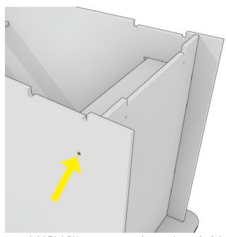
Add BLACK screw to rear brace through right wall as shown.
