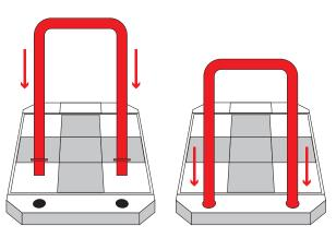
2. Using 2 of the included large lug bolts, securely fasten each bolt into the base of the bar from the **underside** of the stage.
