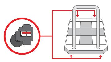
Stabilize the stages from movement and vibrations by loosening the wingscrew and spinning the red tightener on each stage's wheels counterclockwise until the stage is raised off of the wheels and leveled.
