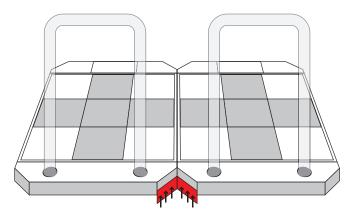
Install the Triangular Cover bracket to the front of the stages in the same way the rear V-bracket is attached with the silver-side upwards. Use 6 M8 screws and lock washers to secure.
