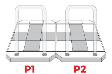
5. Using one of the included **V-brackets** and 6 of the included M8 screws and lock washers, attach the bracket onto the **back** of the stages.
