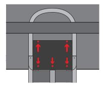
13. Install the front access cover by taking the cover and aligning the 4 mounted screws with the holes along the front hinge, pointed towards the inside of the main unit. Attach the cover by using 4 nuts, one on each screw.
