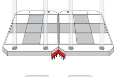
5. After both V-brackets have been installed, fully tighten all 12 screws until they are secured.
