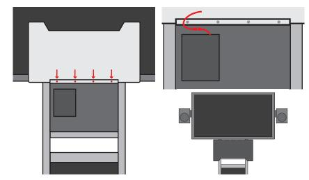
14. Plug the light cable from the cover into the lose plug inside the main unit.
