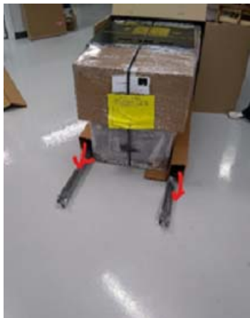
Figure 2.5 Remove Bottom Corner Protectors
