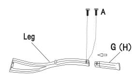
See Page 1 to determine the correct height you wish to assemble your stool. Insert four short feet (G) for counter height or long feet (H) for bar height in to the legs and secure by using short allen bolt (A) as shown
