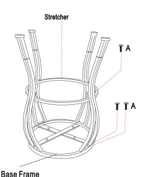
Attach the fourth leg to base frame and stretcher by using short allen bolt (A) as shown
