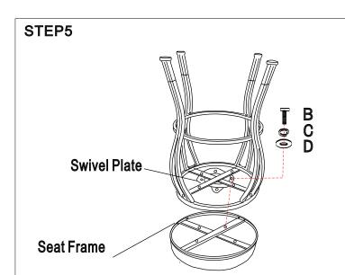
Attach swivel plate (G) to seat frame by using long allen bolt (B), spring washer (C) and flat washer (D) as shown
