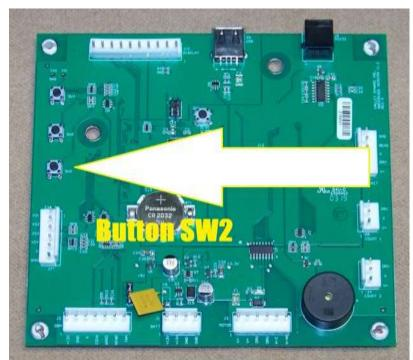
To go into program mode hold down the SW2 switch as the display counts down from 5, release after your display shows
