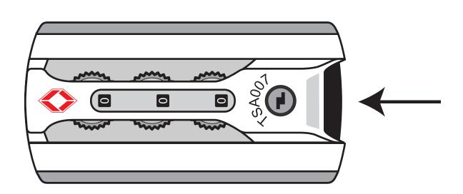
2. Once the suitcase is unlocked and fully opened, locate the switch on the underside of the lock(s).
