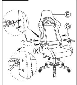
Please be careful to use the correct BLUE Screws (K) and Backrest Screw Caps (G). Insert 4 Screws (K) into the predrilled holes as shown in the diagram above. Tighten securely with the enclosed Allen Wrench (H). Insert 1 Backrest Screw Caps (G) over each of the 4 screws on the Backrest to cover the exposed holes of the Backrest (E).
