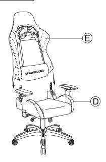
With the two upright bars pointing straight up, lower the backrest (E) onto the two upright bars so they slide into the holes on each side of the backrest. Push down until the connection is secure.
