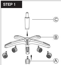
Press the Casters (A) into the hole at the end of each leg of the Base (B). Insert Seat Post (C) into the center hole of the Base (B).
