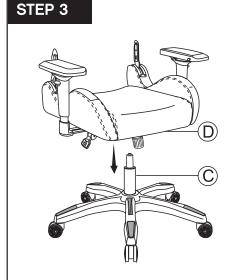
Turn the assembled seat upright and locate the center hole of the Mechanism over the seat post. Push down firmly until the connection is secure.
