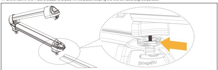
2. Push the red button to the left gently. Pull out the rubber rack and tighten the bolt with the socket wrench of the mounting support to grab the crossbar firmly. Push back the rubber rack and the red button into the original position.
