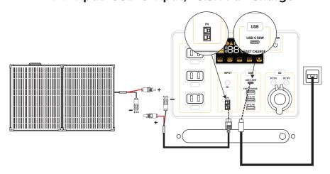
Note: Using USB-C charging can help you shorten the charging time. According to different charging protocols, you can get input power in the range of 0-60W.
