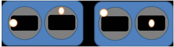
The graphics above show the stick command to bring up the OSD menu. The stick command is: throttle centered, yaw left, pitch forward. The exact stick command therefore depends on which mode your transmitter sticks are in.
