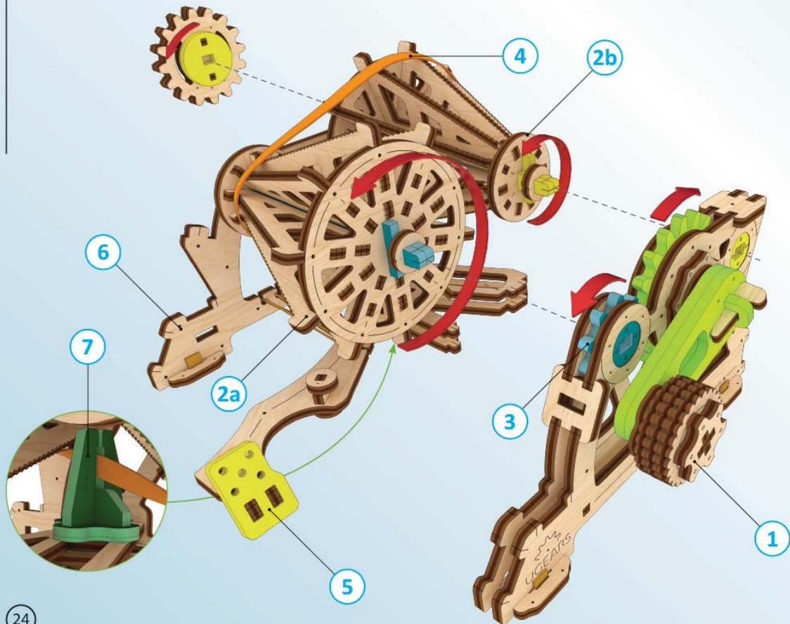
**ENG** Rotating the key (1) initiates the drive cone pulley (2a) via the reducer (3). The belt transfers the rotation to the driven cone pulley (2b). Pushing the pedal (5) attached to the body (6), the transmission fork (7) holding the belt moves, which changes the rotation speed of the driven cone pulley (while the drive cone pulley's speed remains the same).
