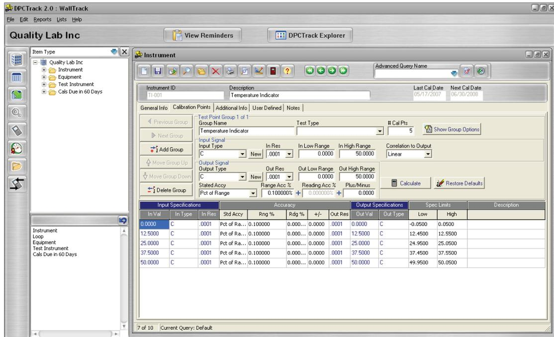
Fluke 750SW DPC/TRACK 2 software includes an instrumentation data-base that makes it easy to manage your instrumentation, create and schedule tests, load and unload the 753 or 754, print a variety of standard reports, and manage calibration data.
