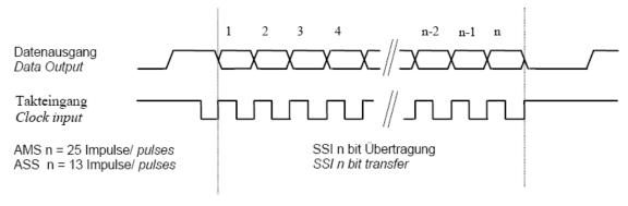
If a new data transfer is started within 20  $\mu$ s, no data reading from the code discs will be made but data of the previous cycle will be transmitted again (data repetition).
