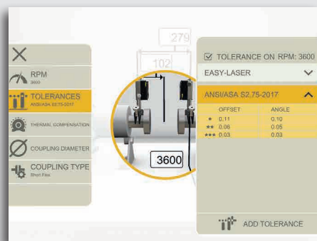
Tolerance check (pre-set or custom)
