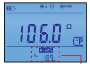
2P mode used for continuity and bonding checks – is active when the instrument is turned on.
