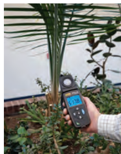
Measure and record multiple measurements to create an illuminance map of the room or area of interest
