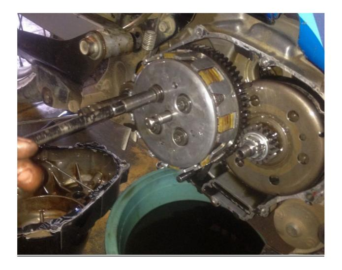
Next step is to insert items in the package to the clutch case. First insert item no.8 from the hole on the top and then item no.6 (seal)
