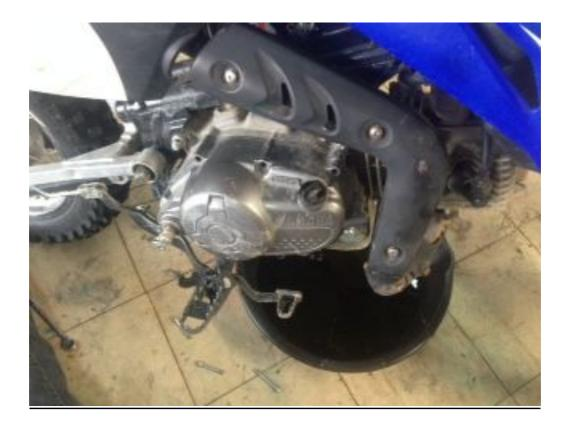
First you need to remove the kick starter, foot pegs (4 bolts under the engine), and the right motor case. Don't forget to drain the motor oil first (bolt on left side of engine).
