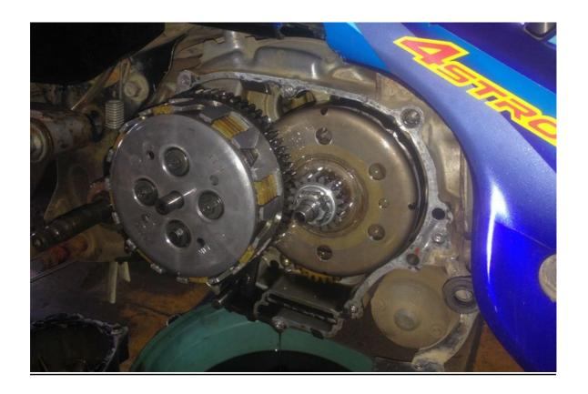
Now remove the clutch house by unscrew 4 bolts and replace the item with circle mark with the ones provided in the package. (item no.2)
