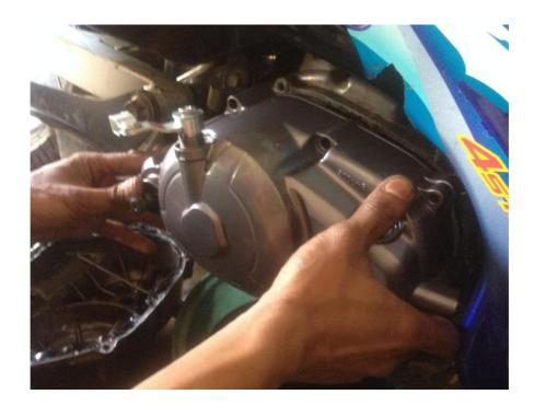
Final step is to put item no.1 and attach the cable just like picture below Then adjust the clutch cable to the handle
