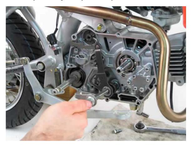
C11. Install the new gearshift spindle assembly. Be sure that the shift shaft seal on the left side of the bike remains in place while inserting the new gearshift spindle assembly.
