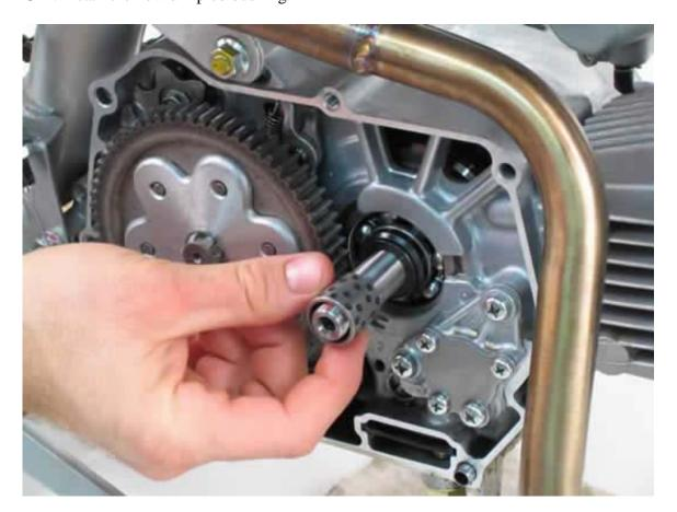
C15. Install the new primary drive gear.
