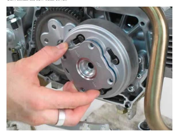
C20. Install the new bearing into the outer cover.
