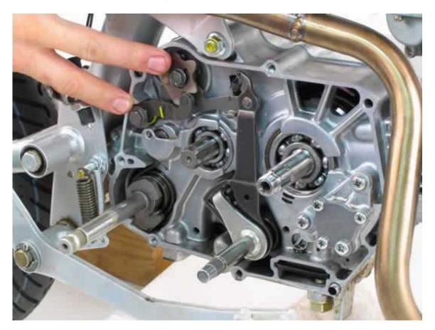
C10. Carefully remove the gearshift spindle assembly.
