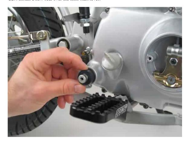
**C28.** Remove the chrome cover plate and remove the Phillips head bolt. Remove the clutch actuator plate assembly. Install the new oil seal. Make sure that the oil seal is completely seated. Replace the clutch actuator plate assembly.
