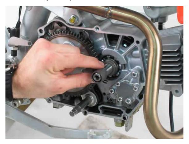
C7. Use snap ring pliers to carefully remove the snap ring. Remove the large driven gear.
