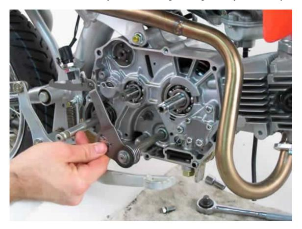
C12. Install the new large driven gear.
