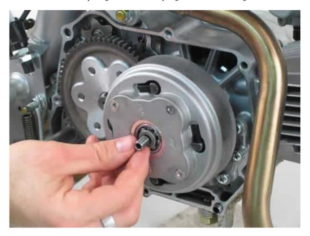
C24. Flip the new clutch cover over and insert the clutch actuator into place (first grease it with water proof grease and try to get it into the seal that it slides into. Same seal as shown in C28)
