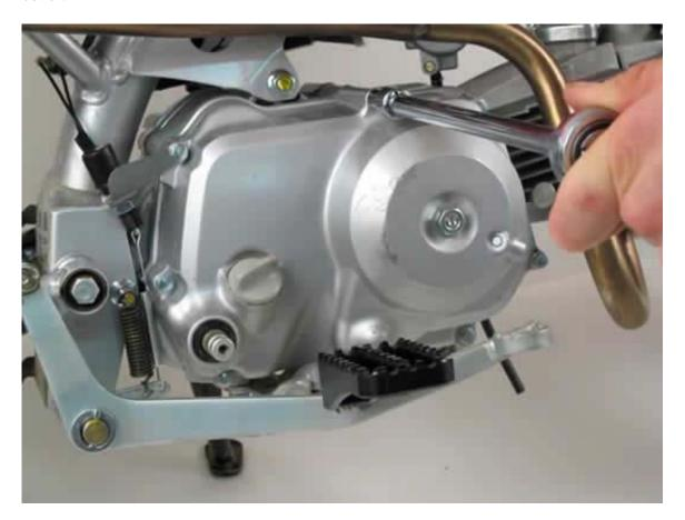
**C3.** Use a Phillips head screwdriver (or in impact driver) to remove the 4 screws from the outer clutch cover.
