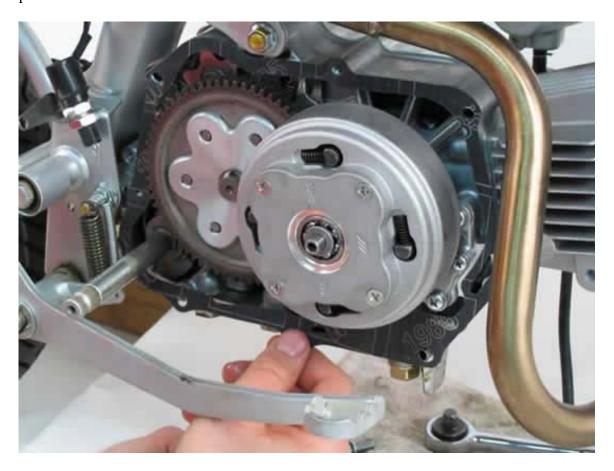
C26. Install the new clutch cover into place and secure with the new Allen head bolts included in the kit.
