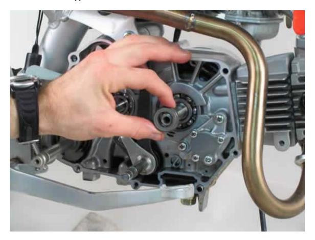
**C9**. Use a 10mm socket to remove the 2 bolts securing the stopper plate and stopper arm. Be sure to pay attention to how the stopper plate and stopper arm line up. (On install, be sure to torque the two bolts and a tiny drop of locate may be a good idea. Be very careful with the lower bolt not to break it).
