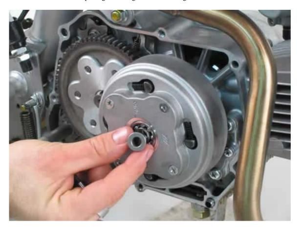
C22. Install the new spring into the bushing.
