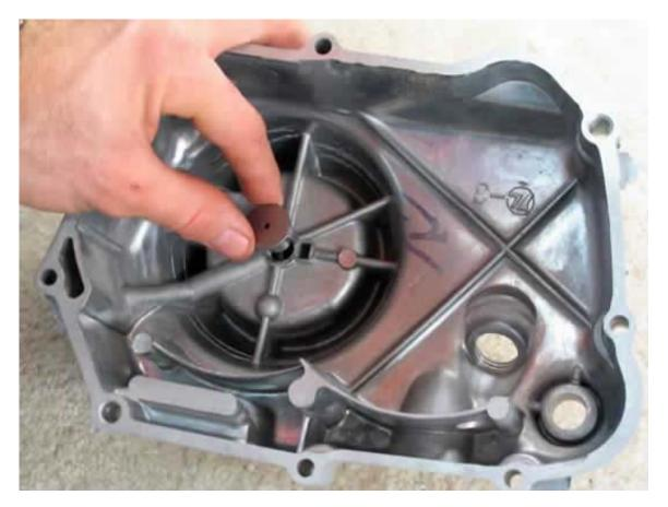
C25. Install the new clutch cover gasket over the two existing dowel pins to keep it in place.
