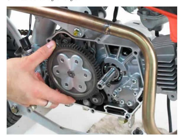
C13. Install the new stepped collar. The tapered portion of the collar should face away from the engine.
