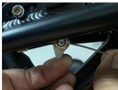
To secure the rear, pull the brake cable arm frontward until it stops. While holding, pull the brake cable rearwards just enough to remove the slack. Then tighten the nut.
