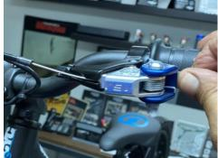
Install the brake cable anchor into the ASV brake lever. Install the ASV brake lever into the perch so that the lever is fully against the perch.
