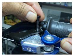
Use the original nut and bolt to secure the ASV lever to the perch.
