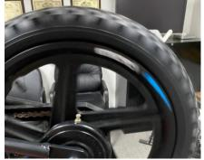
Test the install by spinning the rear wheel. It should spin freely. If struggling, try adjusting at the brake lever before adjusting at the brake cable arm.
