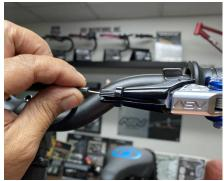
Push the brake cable back into the perch and tighten the brake cable adjustor all the way.
