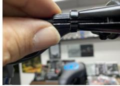
Locate the brake cable adjuster on the brake perch. Use your fingers to loosen the adjuster and line up the openings so that the cable can be removed.
