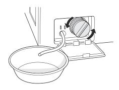
**5** Clean the pump filter and opening.
