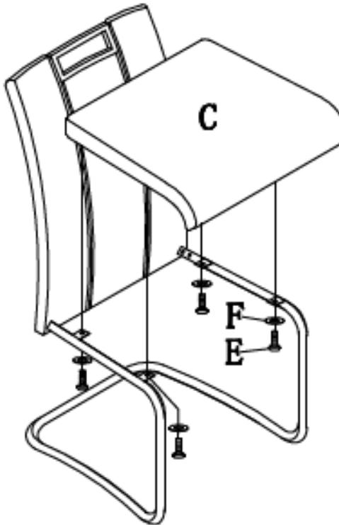
DO NOT TIGHTEN BOLTS UNTIL COMPLETELY ASSEMBLED.
