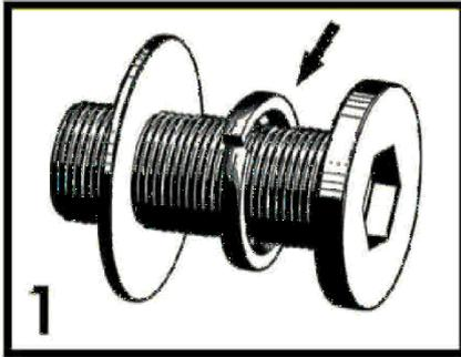
1 Before attaching each of the screws, make sure that the **smaller lock washer is between** the larger washer and the head of the screw.
