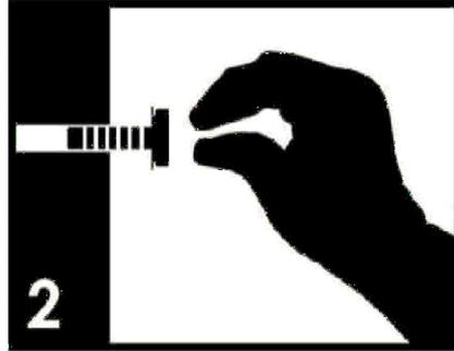
2 Position each part correctly and insert all screws into their respective holes. Then, **hand-tighten** only until 70% tight. Complete tightening with the tools will come at a later step.
