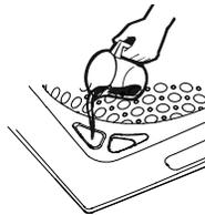
When the **Tank Low** or **Tank Empty** LED is illuminated, more detergent should be added to the reservoir to ensure detergent will be available for the next cycle.
