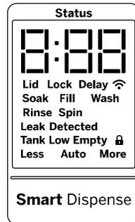
**If it is desired to manually select the amount of detergent for a given load, this can be done by pressing the **Select** button on the **Smart Dispense** control panel to choose between **Less** or **More** detergent. **Less** will provide less detergent than the **Auto** selection and **More** will provide more detergent than the **Auto** selection.**
