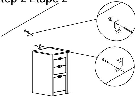
1. Screw the metal bracket into the anchor of wall.
