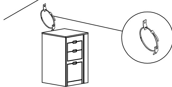
1. Insert strap thru the bracket attached to wall and the second attached to the product.
