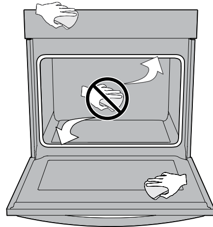
Figure 13: Clean around the oven door gasket
