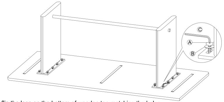
flip the legs on the bottom of wooden top matching the holes to fix the bolts tighten the them as required
