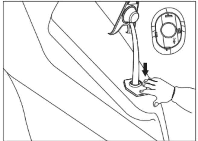
2) Connect the main remote-control cable to the connector under the seat.
