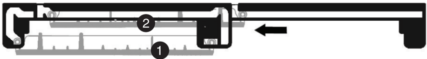
Left rack adjusted to lower position and right rack moved to the left
