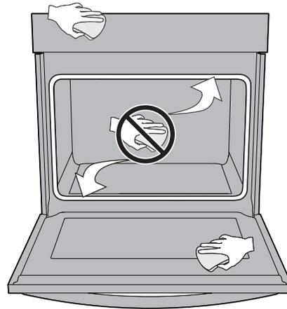
**Figure 13: Clean around the oven door gasket**
