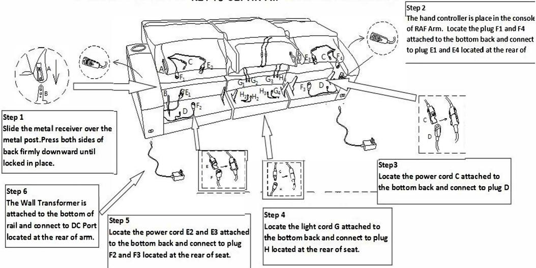
Note: Make sure all PLUGS are connected on the product before plugging power cord into power outlet. If not damage can occur.
