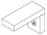
\*After turning the cam lock case to the locked position, the cam lock arrow will be located in the position shown above.
