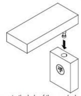
\*Ensure that the cam lock arrow is pointed to the hole, align the cam lock screw to the hole of the cam lock case.
