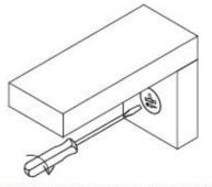
\*Use a straight edge screwdriver to turn cam lock case until it is locked.Locked position is approximately 1/2 turn(210°) clock-wise.
