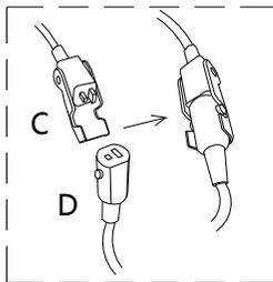
2. Locate the power cord C attached to the bottom back and connect to plug D located at the rear of seat.
