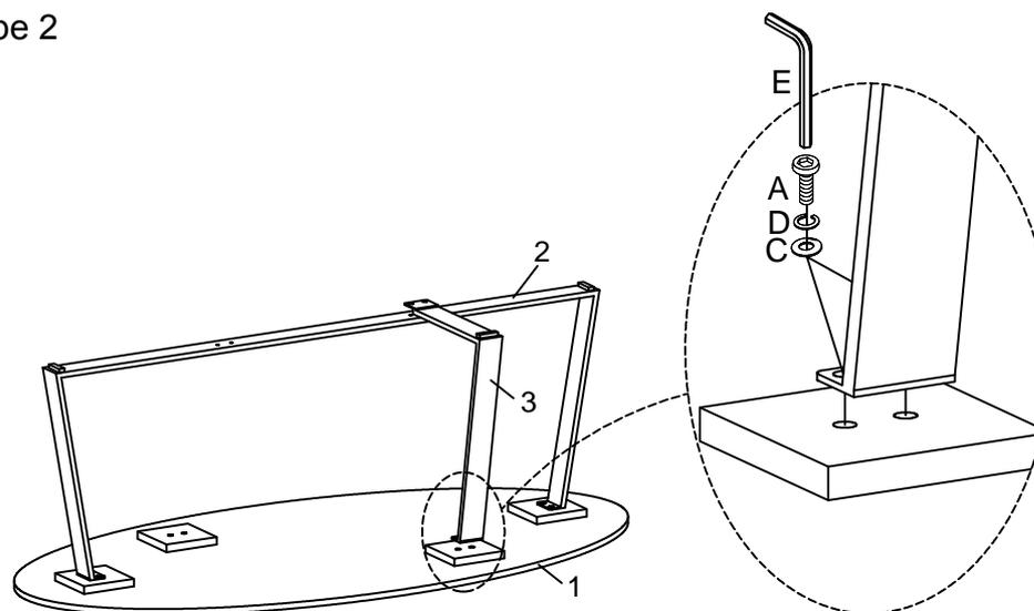
Note: At this stage, do not fully tighten the bolts .
