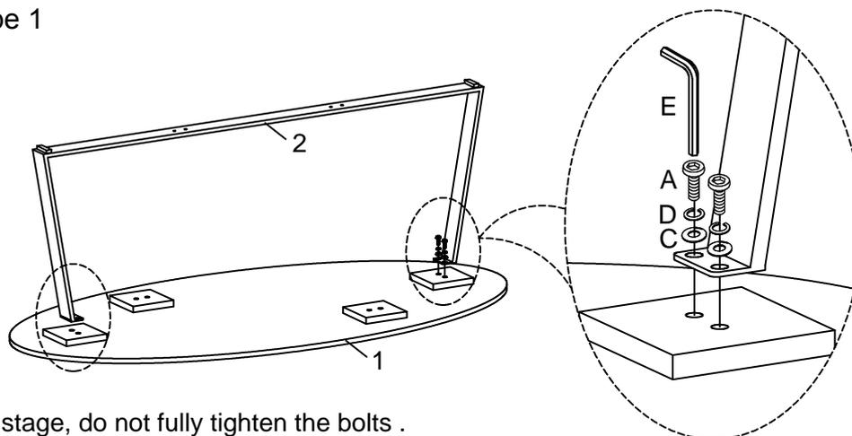
Note: At this stage, do not fully tighten the bolts .
