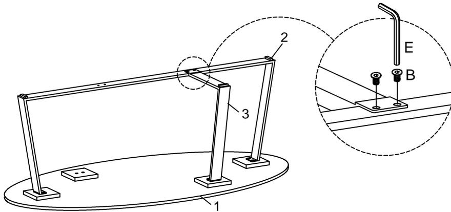
Note: At this stage, do not fully tighten the bolts .
