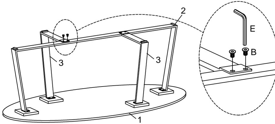
Note: Do not full tighten all bolts until complete assembly.
