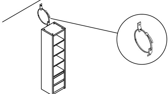
1. Insert strap thru the bracket attached to wall and the second attached to the product.
