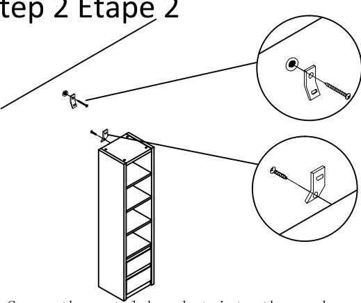
1. Screw the metal bracket into the anchor of wall.
