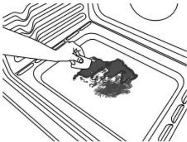
2. Pour distilled or filtered water onto the bottom of the empty oven, and close the oven door.
