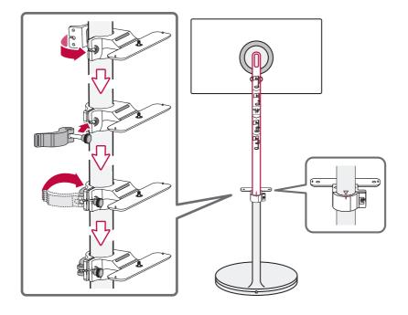
3 Put the speaker on the cradle and turn the screw under the cradle as if pushing it upward to secure the speaker.
