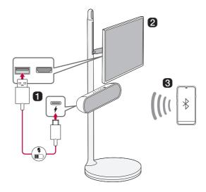
Charge the speaker before using it by opening the rear cover and connect the speaker to the USB port on the StanbyME TV by the USB cable.
