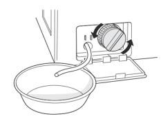
Clean the pump filter and opening.
