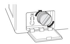
**8** Close the drain pump filter cover.
