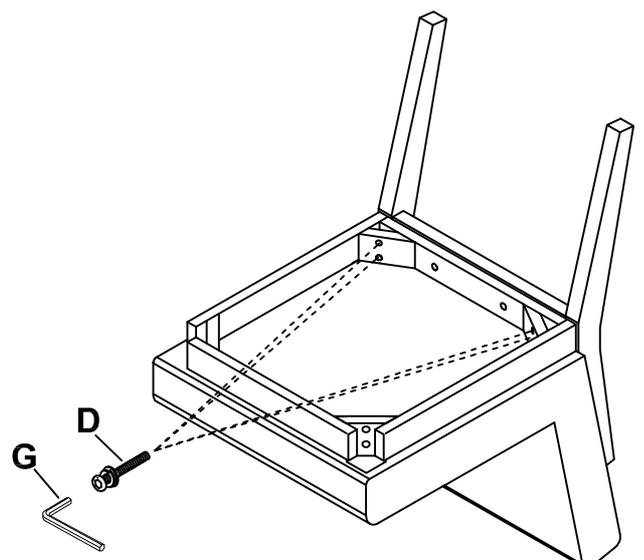
**DO NOT TIGHTEN BOLTS UNTIL COMPLETELY ASSEMBLED.
