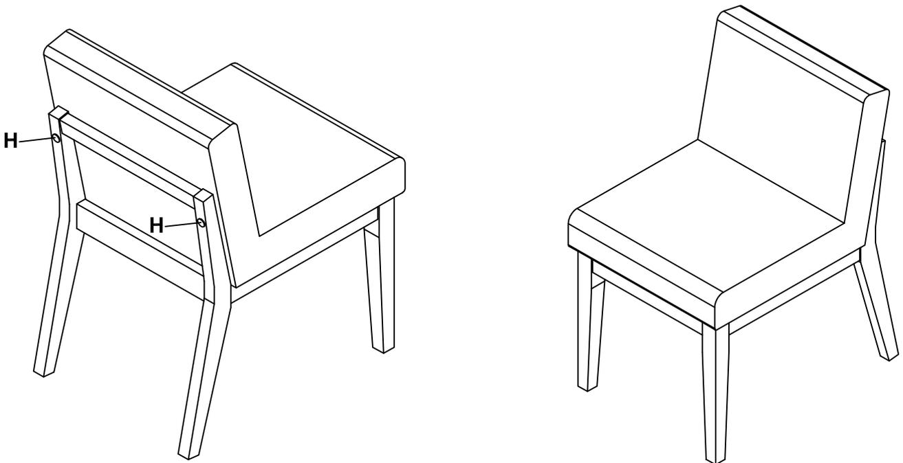
**DO NOT TIGHTEN BOLTS UNTIL COMPLETELY ASSEMBLED.**
