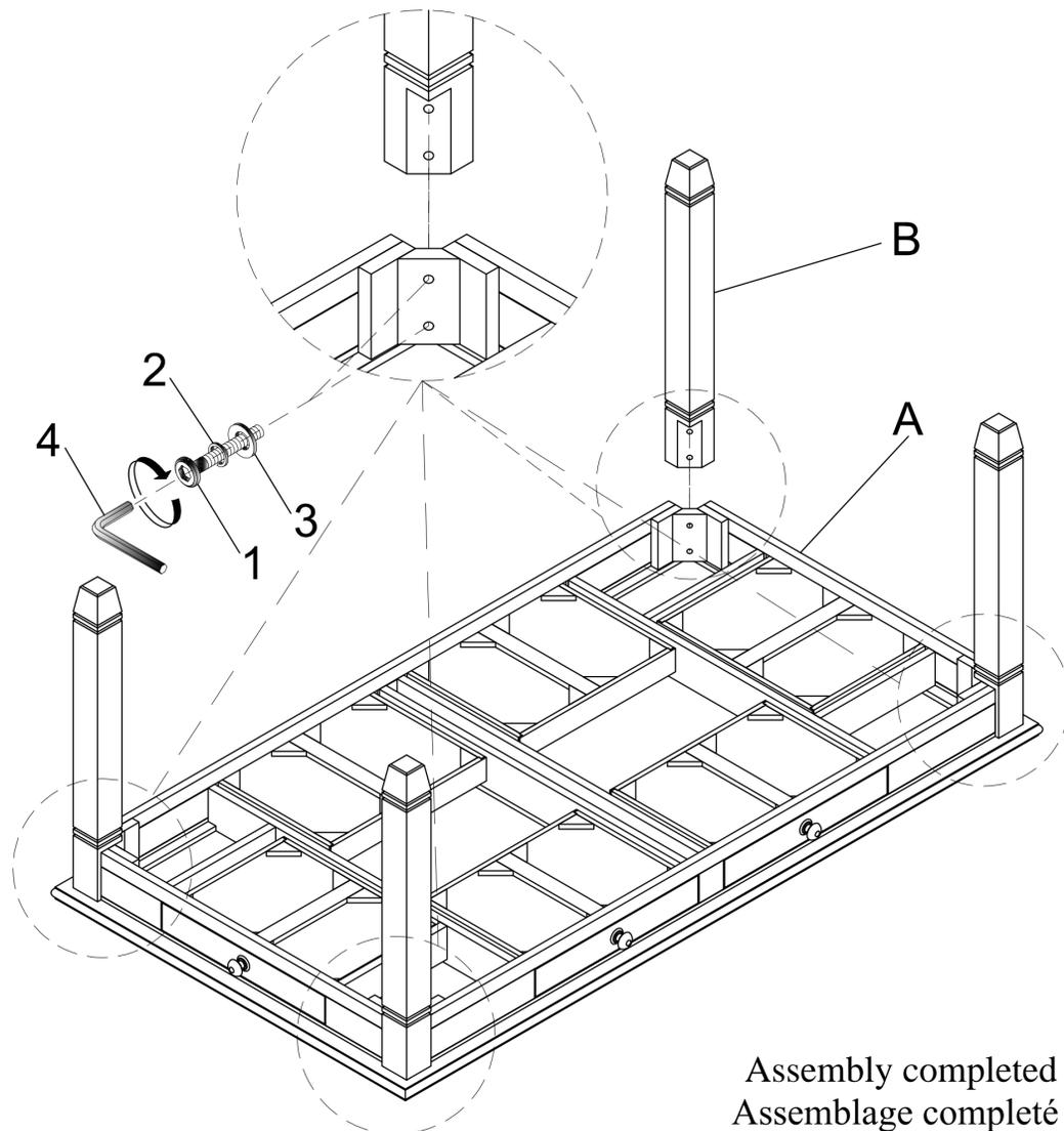
DO NOT TIGHTEN BOLTS UNTIL COMPLETELY ASSEMBLED.
