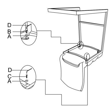
Note: Please do not tighten all bolts until the item is fully assembled. Once assembled tighten all bolts.
