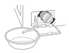
Clean the pump filter and opening.
