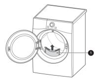
Always ensure that the lint filter is properly installed before running the dryer. Running the dryer with a loose or missing lint filter will damage the dryer and articles in the dryer.
