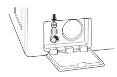
Insert the drain pump filter and twist it clockwise.
