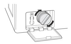
Close the drain pump filter cover.
