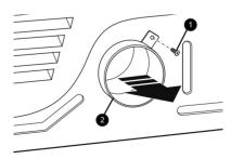
Press the tabs on the knockout 3 and carefully remove the knockout for the desired vent opening. (Right-side venting is not available on gas models.) Press the adapter duct **4** onto the blower housing and secure to the base of the dryer as shown.
