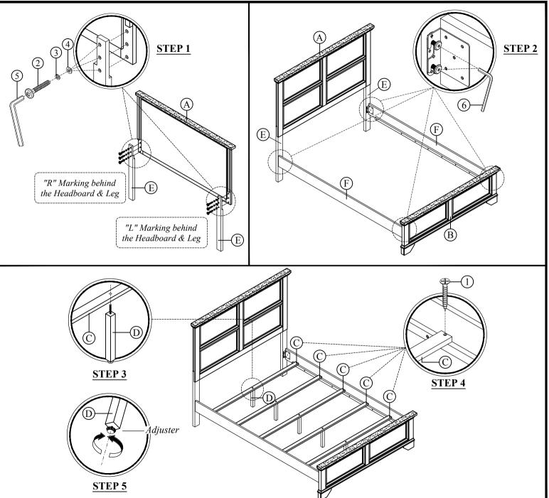
NOTE: MUST TIGHTEN SCREWS PERIODICALLY. SCREWS NATURALLY LOOSEN WITH USE. CHECK TIGHTNESS OF ALL SCREWS EVERY 6-8 WEEKS.
