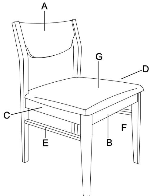
Do not tighten bolts until completely assembled.
